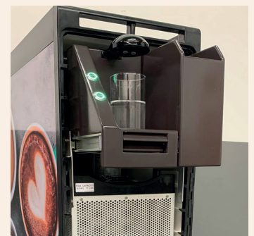
Dispensing head and storage container pulled into outward position for service
